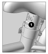
Push in the battery safety button to turn the power on.
