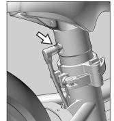
Ensure the cable is securely connected before operation. A loose connection can result in faulty operation of bike.
