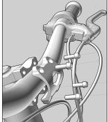
Install handlebar. Use a 4mm Allen wrench tighten the 4 screws to 3.75 ft lbs (IMPORT-ANT- DO NOT OVER-TIGHTEN). The brake lever should be on the brake side of the bike.
