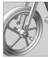
Attach the front wheel. Use a 15mm wrench to tighten the axle bolts to 12.5 ft lbs (IMPORTANT- DO NOT OVER-TIGHTEN). An improperly installed front wheel may cause accidents and injuries.
