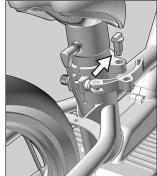
Adjust seat height. Remove the latch screw to open the latch. Make adjustments. After adjustments, close the latch and put the screw back in. The latch might need to be rotated to get the right clamping power.
