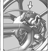
Inspect the brake to make sure it produces adequate stopping power. Adjust the cable tension nut to control brake free play if needed.
